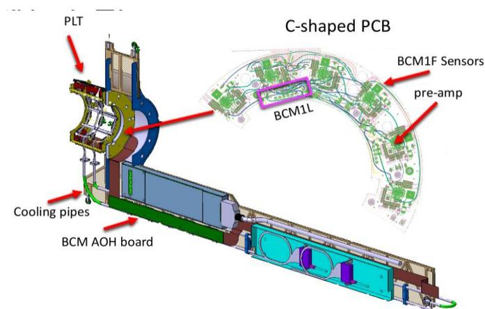
*Figure 1 A sketch of the frame where PLT and the BCM1F sensors are placed*
