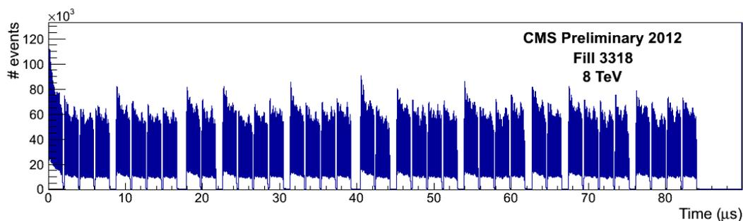
Figure 4 Counts as function of orbit-time for the determination of the bunch-by-bunch luminosity.
