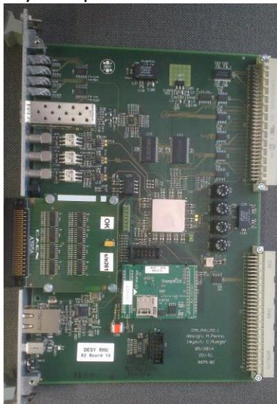
Figure 3 The RHU histogramming unit
