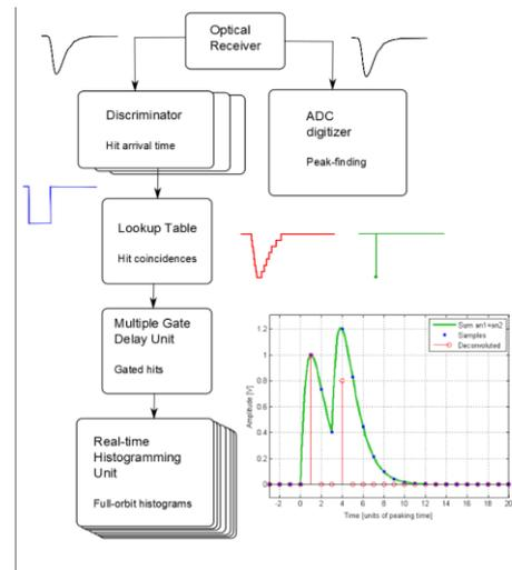
Figure 2 The two streams of the readout for BCM1F
