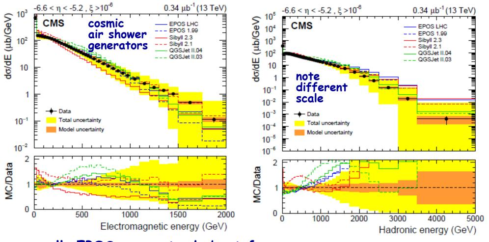
overall, EPOS seems to do best for electromagnetic ( $\pi^0$ ) and hadronic ( $\pi^{\pm}$ ) energy fractions
