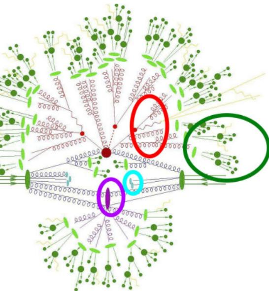
A  $p\bar{p}$  collision at the LHC can be interpreted as a **hard scattering** between partons accompanied by *underlying event* (UE) consisting of:
