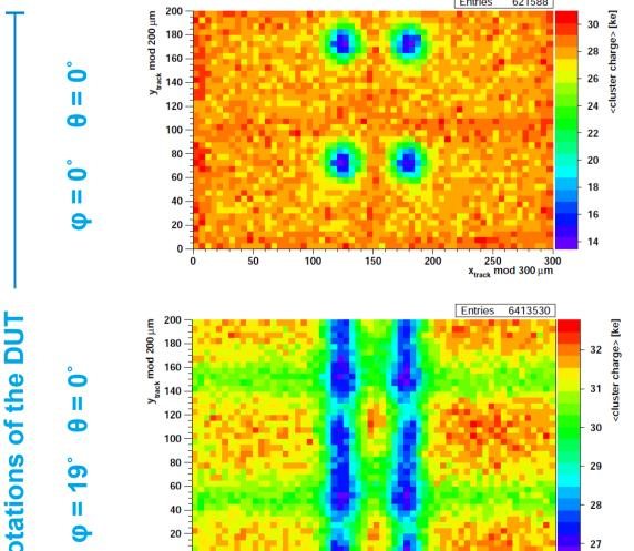
The high resolution of the beam telescope tracks have been used to study various effects within single pixel cells of the CMS Pixel sensor at different incidence angles.
