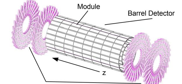
The modules of the CMS Pixel detector hold one sensor and 16 ROCs. Special single-ROC modules are produced for test purposes such as laboratory measurements or test beams.
