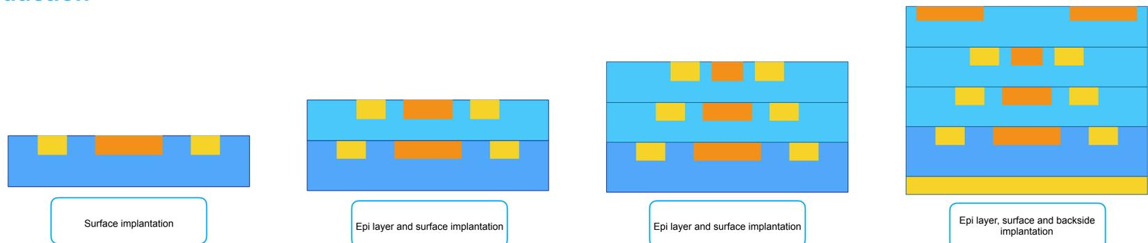
The first stage of production is p and n surface implantation. Implantation is done by bombarding the wafer with an ion beam of defined energy. After first-time surface implantation wafer is polished and prepared for epitaxial silicon growth.
