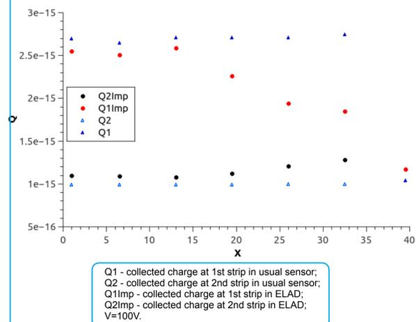
The collected charge as a function of the MIP incident position is shown. The x-axis - position of MIP [μm], the y-axis - collected charge [C]. The plot shows that the ELAD detectors have better charge sharing (red and black dots) than the usual design detectors (blue and light blue triangles).
